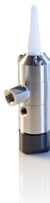
**Fluid Inlet Port:** 3/8" NPT Female**Fluid Outlet Port:**  $\frac{1}{4}$ " NPT Female**Aux Air Inlet Port:** 1/8" Female**Min Air Pressure:** 70 psi (4.8bar)**Max Fluid Pressure:** 2500 psi (172.4bar)**Mounting Port:** N/A**Viscosity Range:** 1- 3 000 000cps**Wetted Parts:** 303 SS, hard Chrome plated stainless steel, UHMWPE, EPR**Operating Frequency:** 400+ cycles/min
